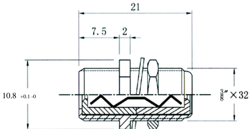
Corps moulé ( alliage Zinc ) / Body in Die Cast ( Zinc Alloy )
